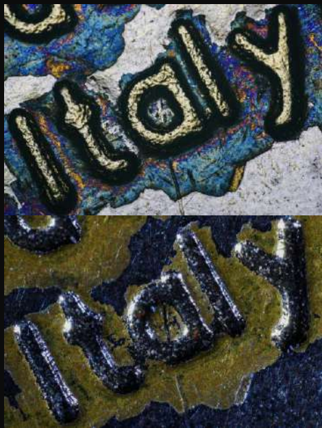
Coaxial light (Top) & Normal lighting (Bottom)
