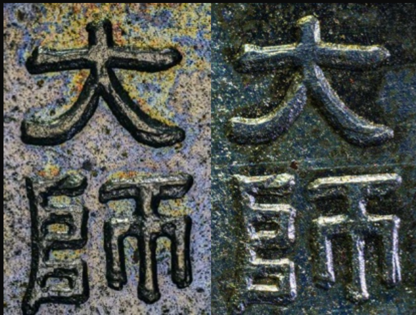
Coaxial light (Left) & Normal lighting (Right)
