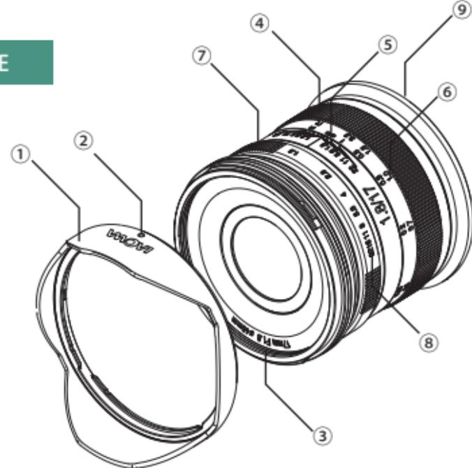
①: Lens hood ②: Lens hood mounting index ③: Filter thread
